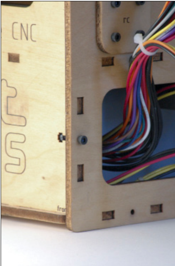
Bolted tenon or T-slot joint.
