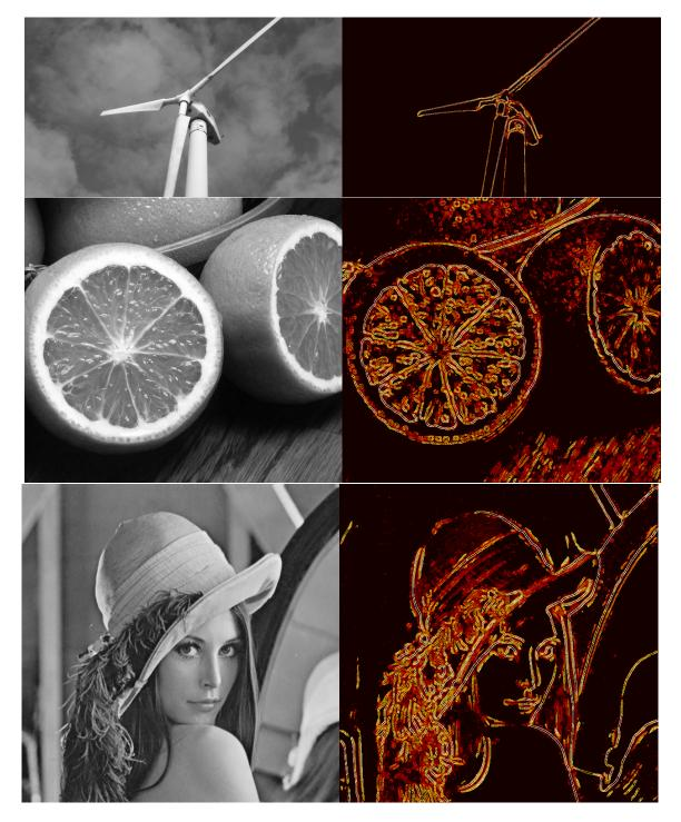
Figure 25: Effect of the  $\sigma$  parameter for the *Marr-Hildreth* (Gaussian) algorithm on our sample images. For each example we show the original image on the left and the generated saliency map on the right.  $\sigma$  is sampled regularly in the range [0.5, 5] using a step of 0.5.
