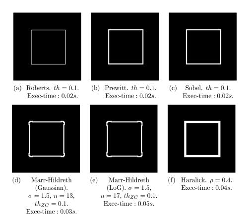
Figure 13: Results of the algorithms using Figure 12 as input image. The first three ((a), (b) and (c)) correspond to the first derivative methods (Roberts, Prewitt and Sobel), then the following two ((d) and (e)) are from the Marr-Hildreth algorithm using Gaussian and LoG kernels, and the last one ((f)) corresponds to the Haralick algorithm. Note the rounded corners on the Marr-Hildreth results, due to the Gaussian blur.
