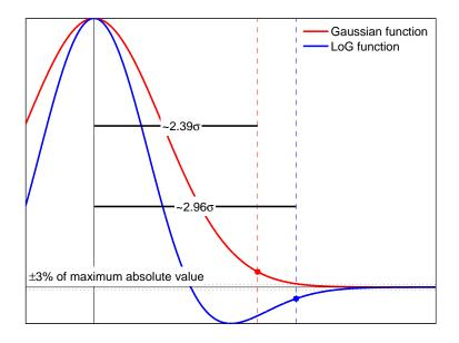
Figure 11: Comparison of the Gaussian and LoG functions.
