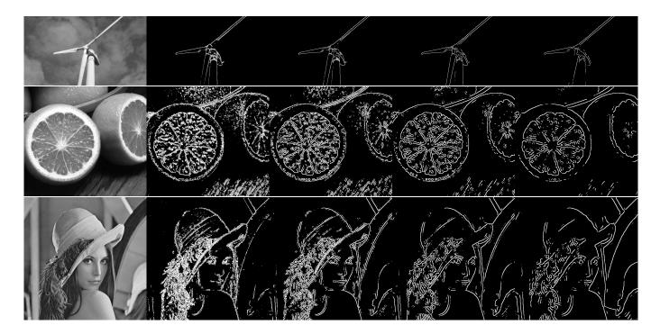
Figure 24: Effect of the  $\sigma$  parameter for the *Marr-Hildreth* (Gaussian) algorithm on our sample images. For each example we show the original image on the left and various consecutive results with different smoothing values ( $\sigma = 1, 2, 3, 4$ ) on the right.
