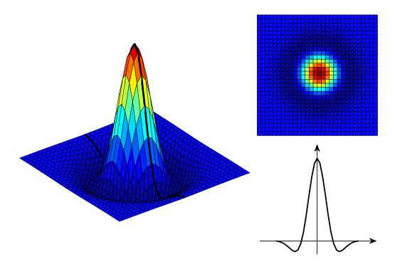
Figure 10: Laplacian of a Gaussian kernel,  $\sigma = 4$ , n = 31. The selected value of n is sufficient to have a good approximation of the LoG function in the kernel, but it is greater than in the case of the Gaussian kernel.
