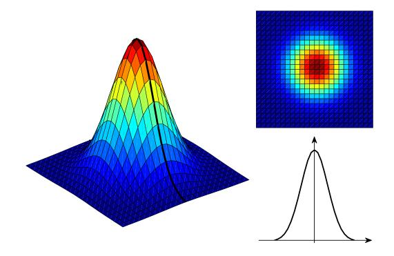
Figure 9: Gaussian kernel,  $\sigma = 4$ , n = 25. It is easy to see that the selected value of n is large enough to have a good approximation of the Gaussian function in the kernel.
