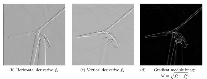
Figure 6: Example computation of the gradient. Original image and gradient image computed using Sobel operators (operators in Figure 5).
